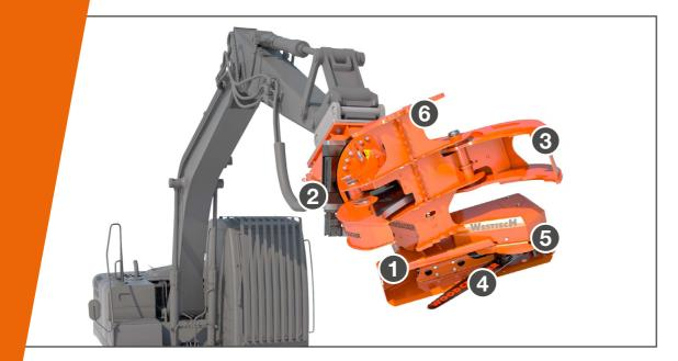
1 Spring-mounted **saw box** prevents the saw blade bending due to force acting on it.
